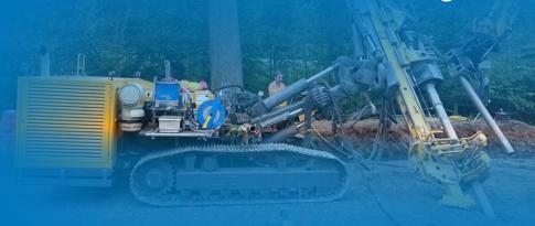
The Water-Propelled **Down-The-Hole Hammer**
