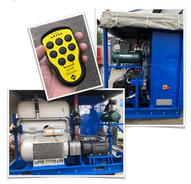
\*Pump capacity is 425l/min@180 bar and 465 l/min@160 bar.
