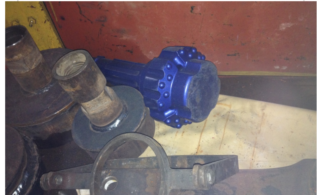
Ø165, Ø224, Ø276 and Ø324 mm reamer bits/hole openers with bit shank DHD350, that were used in the Boliden-Garpenberg mine 2014-16 (Project Case)
